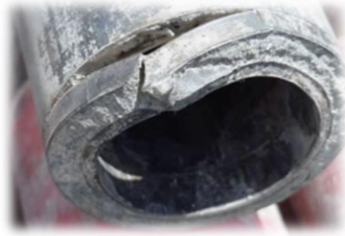
Sour Corrosion ( H 2 S Corrosion)
