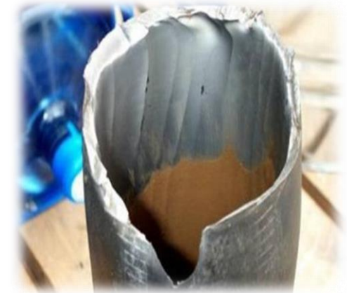
Stress Corrosion Cracking
